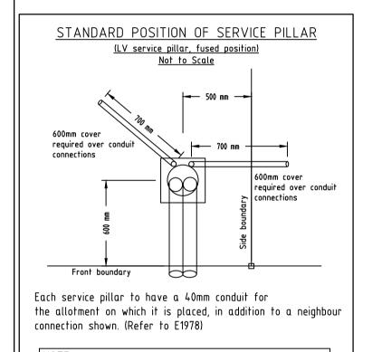
With approval from the relevant SA Power Networks manager, the developer can request a non-standard service pillar position.
