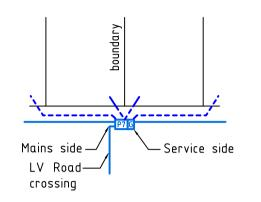
The pit may be offset to avoid a driveway by aligning the short side of the pit with the shared side boundary of the property. The mains and service side can be on either the left or right to suit the site installation.
