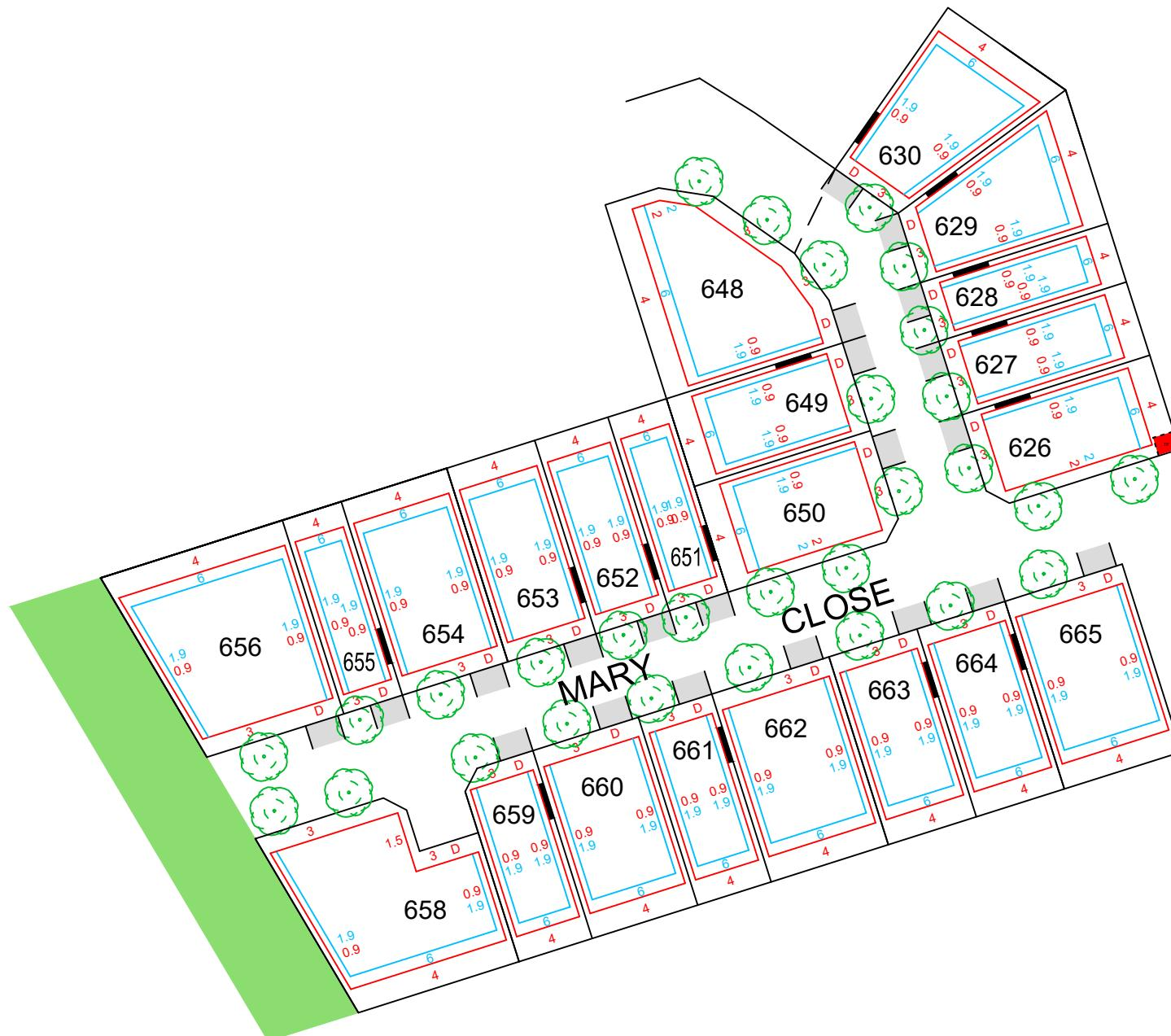
Envelopes are indicative showing minimum set backs only at the time of preparation. Council and Development Plan requirements must also be adhered to.
