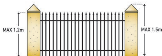
RENDERED MASONRY WITH RAILING
