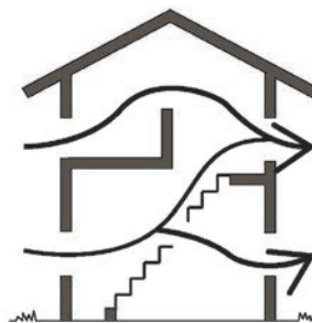
Strategically locating doors & windows during the design phase of your home can promote good conditions for cross-ventilation
